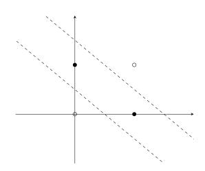
We need two lines to separate this data! A perceptron will never reach the optimal solution. However, multiple perceptrons can learn multiple lines, which can be used to classify non-linearly separable data.
