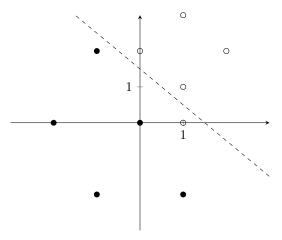
The perceptron that represents the dashed line y + x - 1.5 = 0 has two inputs,  $x_1, x_2$ , with corresponding weights  $w_1 = 1, w_2 = 1$ , and bias b = -1.5. Let y represent the output of this perceptron. In the data above, the point (1,0) is the only misclassified point. The perceptron outputs 0 because it is below the line, but it should output a 1.
