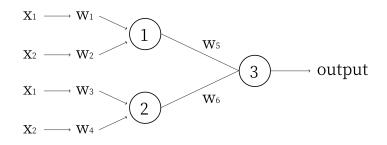
Let perceptron 1 model y + x - 1.5 = 0 (the upper line), and perceptron 2 model y + x - 0.5 = 0 (the lower line). Because the weights are the coefficients of these functions,  $w_1 = 1, w_2 = 1, w_3 = 1, w_4 = 1$  and the biases  $b_1 = -1.5$  and  $b_2 = -0.5$ .
